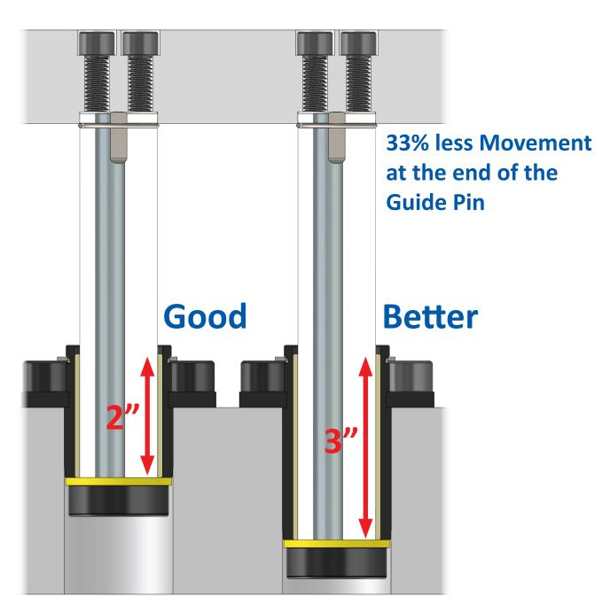
A longer bushing provides more surface area contacting the guide pin which extends the performance life of the Guided Keeper.
