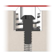
Make sure pocket depth is machined so the travel of the assembly is limited to be equal to, or less than, the max travel.
