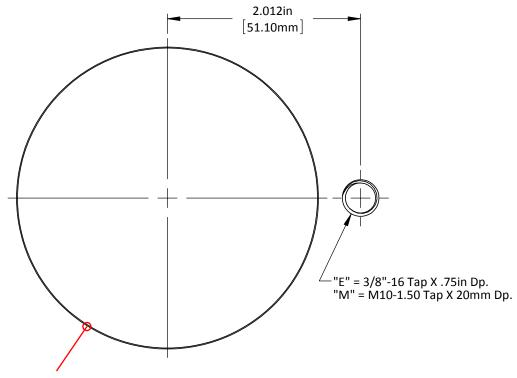
\*Recommended Minimum Hole Size to be Cylinder Body Diameter +1mm [.04"]
