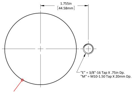
\*Recommended Minimum Hole Size to be Cylinder Body Diameter +1mm [.04"]
