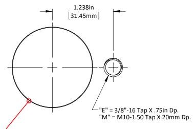
\*Recommended Minimum Hole Size to be Cylinder Body Diameter +1mm [.04"]
